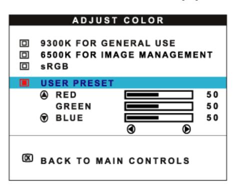
6a) If USER PRESET is highlighted, press the objection to highlight RED. Next, press the objection
